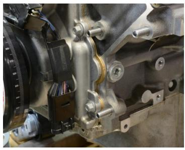
1. Install three M10 x 40mm set screws into the lower driver side of the engine block. Apply Loctite to the threads and tighten, leaving 1/2" of the threads sticking out.
