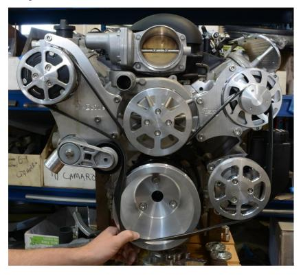
1. Route the belt onto the pulleys as shown installing over the crank pulley last.
