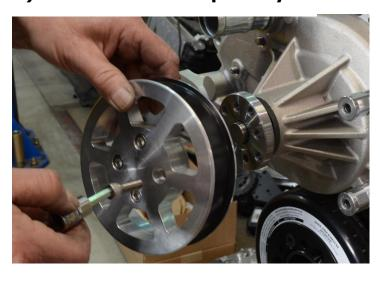
Install the water pump pulley using four  $5/16-24 \times 1$ " cap screws. Apply Loctite to the threads and tighten fully while using caution to prevent over torqueing.
