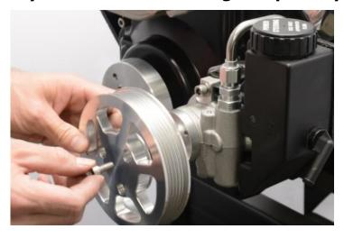
Apply a small amount of Loctite to the three  $1/4-20 \times 5/8$ " cap screws provided and install the power steering pulley. Tighten fully while using caution not to over torque.
