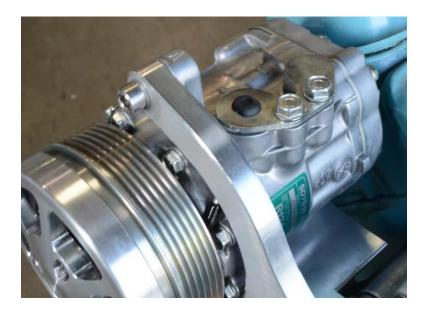
1. Remove the plate from the top of the compressor body. The compressor is charged with Nitrogen to insure lubrication of all components during transport. You will hear the gas escaping when you loosen the fasteners.
