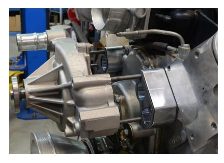
4. Install the water pump over the studs.
