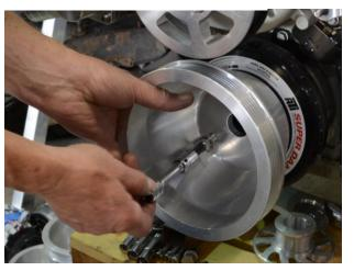
Install crank pulley using three  $3/8-16 \times 1-1/4$ " cap screws and Belleville washers. Apply Loctite to the threads and tighten fully while using caution not to over torque.
