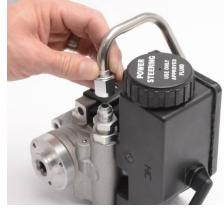
1. If you purchased our kit with a power steering pump with an attached reservoir, install the pressure fitting and hard line onto the pump and tighten them both.
