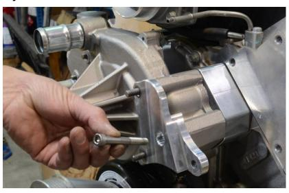
1. Install the rear alternator bracket over the driver side studs and secure with one M8  $\times$  140mm socket cap screw. Tighten this bolt fully while using caution to prevent over torqueing.
