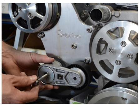
1. Install the tensioner on the A/C bracket using the  $3/8-16 \times 2$  1/4" hex head bolt. Apply Loctite to the threads and tighten fully while using caution not to over torque.
