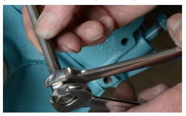
1. Install three M8 studs x 140 mm with anti seize to the passenger side of the block. They should stick out 4-1/2". Use the double nuts provided to help with the install if needed.
