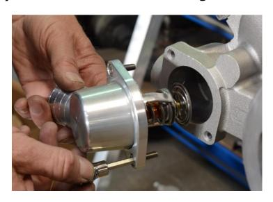
1. Place the thermostat into the housing and install onto the water pump with two M6 x 16mm socket cap screws. **NOTE: After** rotating the thermostat housing to its final installed position, it is imperative that you place the locating tab on the termostat in the approximate index notch on the housing so that the air bleed valve is installed facing "up," as close to the 12 o'clock position as possible. Failure to do so could cause overheating. **SEE BELOW**
