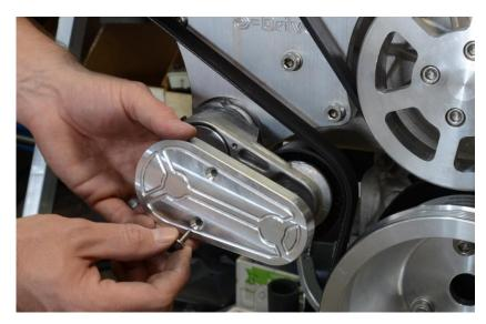
3. Install the aluminum tensioner cover using two 10-32 x 3/4" socket head flat head screws. Tighten fully while using caution to prevent over torqueing.
