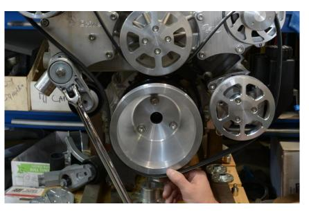
2. Using a 1/2" drive breaker bar, rotate the tensioner down and finish installing the belt around the crank pulley. Slowly release the tensioner until it rests against the belt and tensions the system. **NOTE: In order to achieve an optimum operating position for the tensioner, some applications may require a belt length that appears to be too short and will be difficult to install.**
