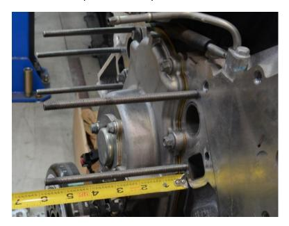
2. Install two M8 studs x 165 mm with anti seize to the driver side of the block. They should stick out 5-3/4". Apply a thin coat of RTV sealant to both sides of the gaskets and install them over the water pump studs.
