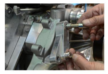
1. Attach rear compressor bracket to the passenger side of the water pump using two M10 x 20mm cap screws with anti-seize. Fully tighten these bolts using caution to prevent over torqueing.
