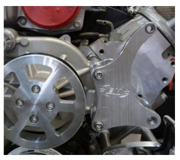
Install the alternator bracket to driver side stand-offs with two M8  $\times$  25mm cap screws and AN washers; leave finger tight. Make sure to use anti-seize on the threads.
