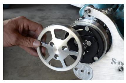
Apply Loctite to the threads of the three  $1/4-20 \times 3/4$ " socket cap screws and install the compressor cover against the compressor pulley. Tighten fully using caution not to over torque.
