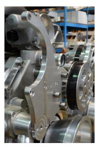
Using anti-seize, install the A/C compressor bracket using three M8  $\times$  25mm cap screws with AN washers. Leave finger tight at this time. **Note: Make sure you have already installed the thermostat and housing before mounting this bracket.**
