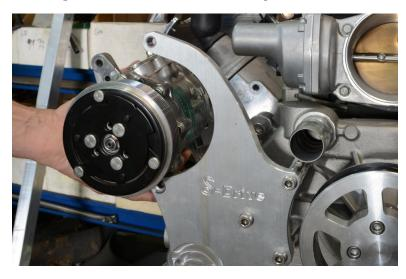
1. Install the A/C compressor using two M8 x 25mm cap screws and leave finger tight for now.
