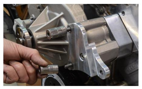
2. Using anti-seize, install two  $3/4 \times 1.41$  stainless steel standoffs to the driver side studs. Do not fully tighten at this time. The end of the stand-off with the hex closest to it goes AWAY from the engine.
