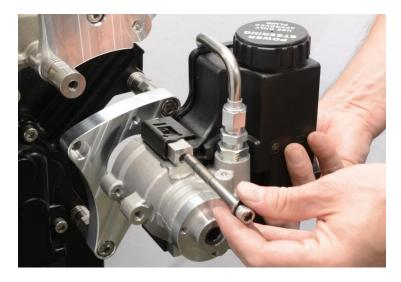
2. Install the pump onto the power steering bracket using two 5/16-18 x 3" socket cap screws and lock washers. Tighten fully while using caution to prevent over torqueing.
