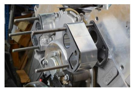
3. Install both of the water pump spacers over the studs (one on the driver side and one on the passenger side) along with another set of water pump gaskets. Apply a thin coat of RTV sealant to both sides of the gaskets.
