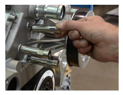
1. Using anti-seize, install three  $3/4 \times 2.55$  stainless steel stand-offs to the passenger side studs. Do not fully tighten at this time.
